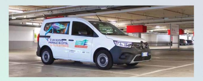
The Cargo service has 100% electric Kangoo Van E-Tech vehicles: compact vans capable of offering a load volume of 3.3 cubic meters thanks to the 45kWh lithium-ion battery, capable of guaranteeing autonomy between the 250 and 300 km. The choice of these vehicles also brings with it a further environmental advantage: when the vehicles reach the end of their life cycle, the traction batteries are reused for the storage of renewable energy.
